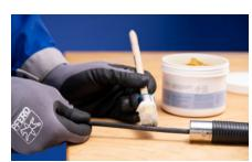
Then apply new special shaft grease to the core.
