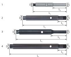
With drive spindle extensions, shanks of grinding and milling tools can be extended. They allow access to difficult-to-reach areas. The extensions are clamped into the collet of the machine (air or electric grinder) or into the flexible shaft handpiece.
