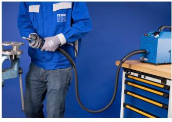
Flexible shaft drive set up incorrectly: flexible shaft bent on the motor side and/or handpiece side.
