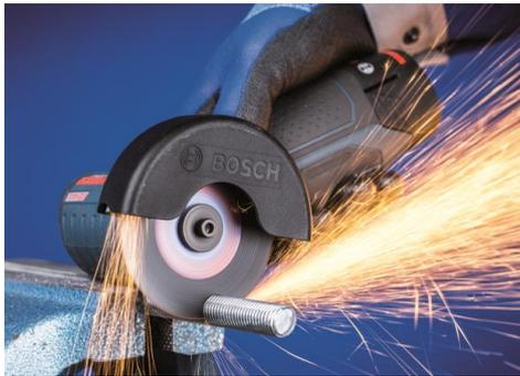
***PFERD presents cut-off wheels in widths of 0.8 und 1.0 mm, which were specially designed for the new compact angle grinders for discs and wheels with a diameter of 76 mm***
